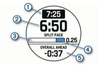
The device displays your target split pace ①, current split pace ②, completion progress for the split ③, distance remaining in the split ④, and overall time ahead or behind of your target pace ⑤.
